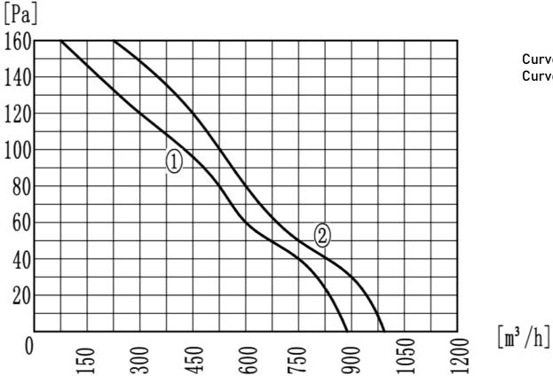
Curve 1: 50HZ Curve 2: 60HZ
